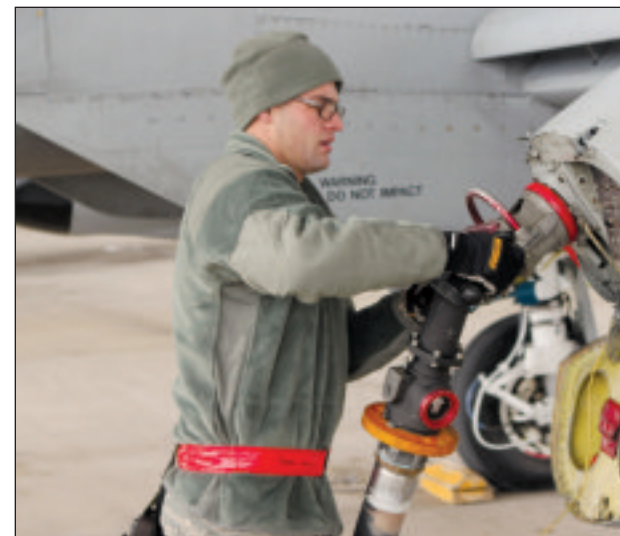
Staff Sgt. Thomas Bourke, a crew chief with the 127th Maintenance Group, refuels an A-10 Thunderbolt II.
